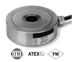
The fully welded constuction and glass-to-metal cableentry ensure that this product can be used successfully in harsh environments found in the food, chemical and allied process industries.
